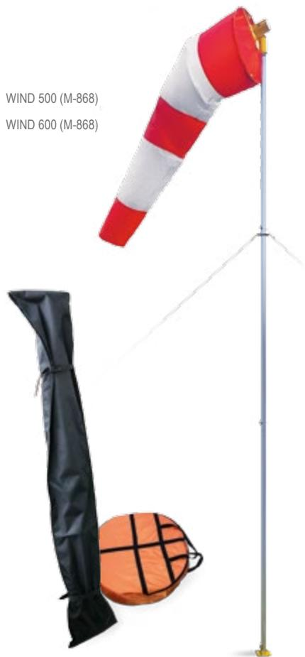
Designed for rapid deployment in the field in light and dark time of day. The construction of the mast is made of aluminum for easy transportation, quickly demountable, three-sectional, with the case for carrying. It is installed both on concrete as well as on the ground surface.
